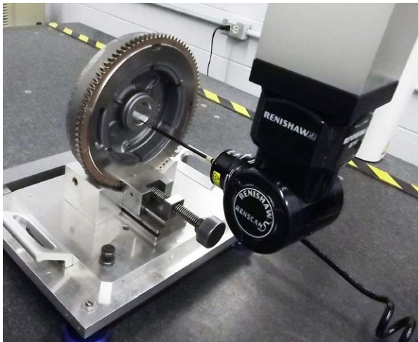
REVO head inspecting a FX series small engine flywheel
